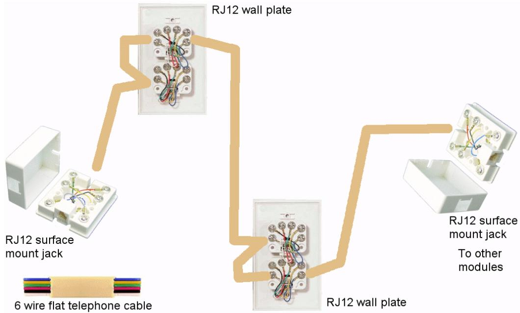
Figure 10: Wiring path for command bus using RJ12 surface mount jacks, walls plates and 6 wire flat telephone cable. No soldering or crimping required.
