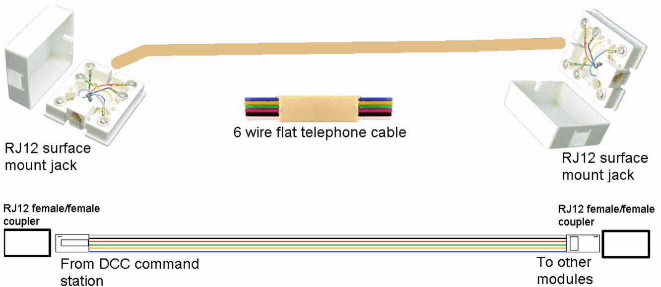
Figure 14: Wiring options for short modules without throttle jacks.
