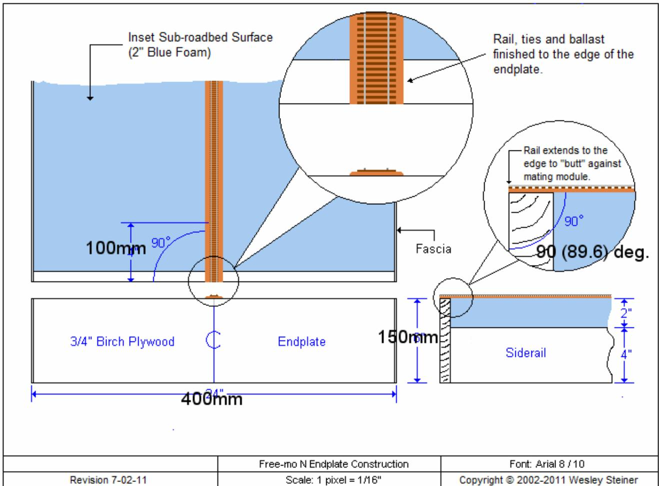
Figure 3: Insert diagram of end plate profile & tolerance, above is place holder example
