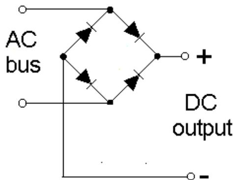
Figure 17: Unregulated full wave rectifier
