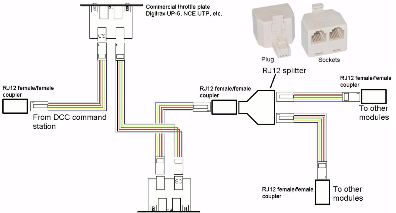
Figure 13: Wiring path for DCC command bus on junction module using commercial throttle jacks, modular telephone components and RJ12 patch leads.
