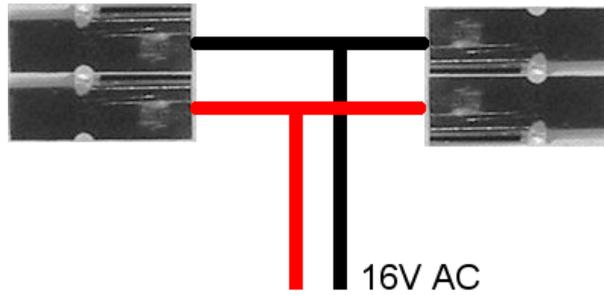
Figure 16: "T" joiner to power AC accessory bus.
