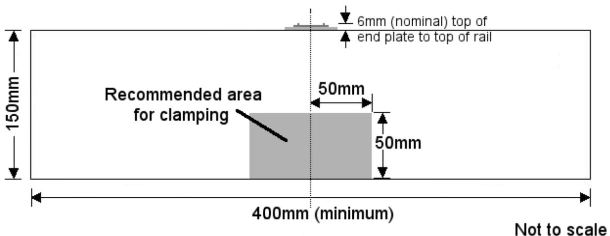
Figure 2: End plate dimensions
