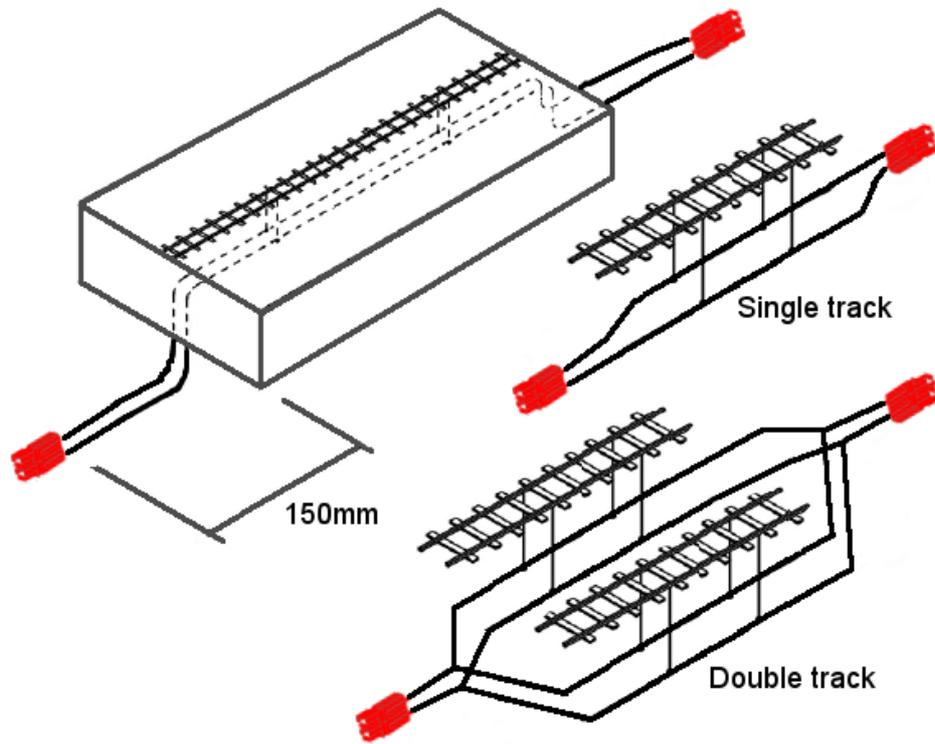
Figure 7: Basic track wiring.
