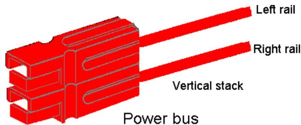
Figure 6: Arrangement of power bus connectors.
