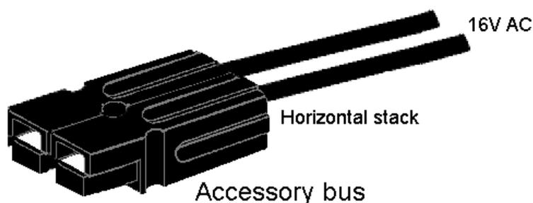
Figure 15: Arrangement of accessory bus connectors.
