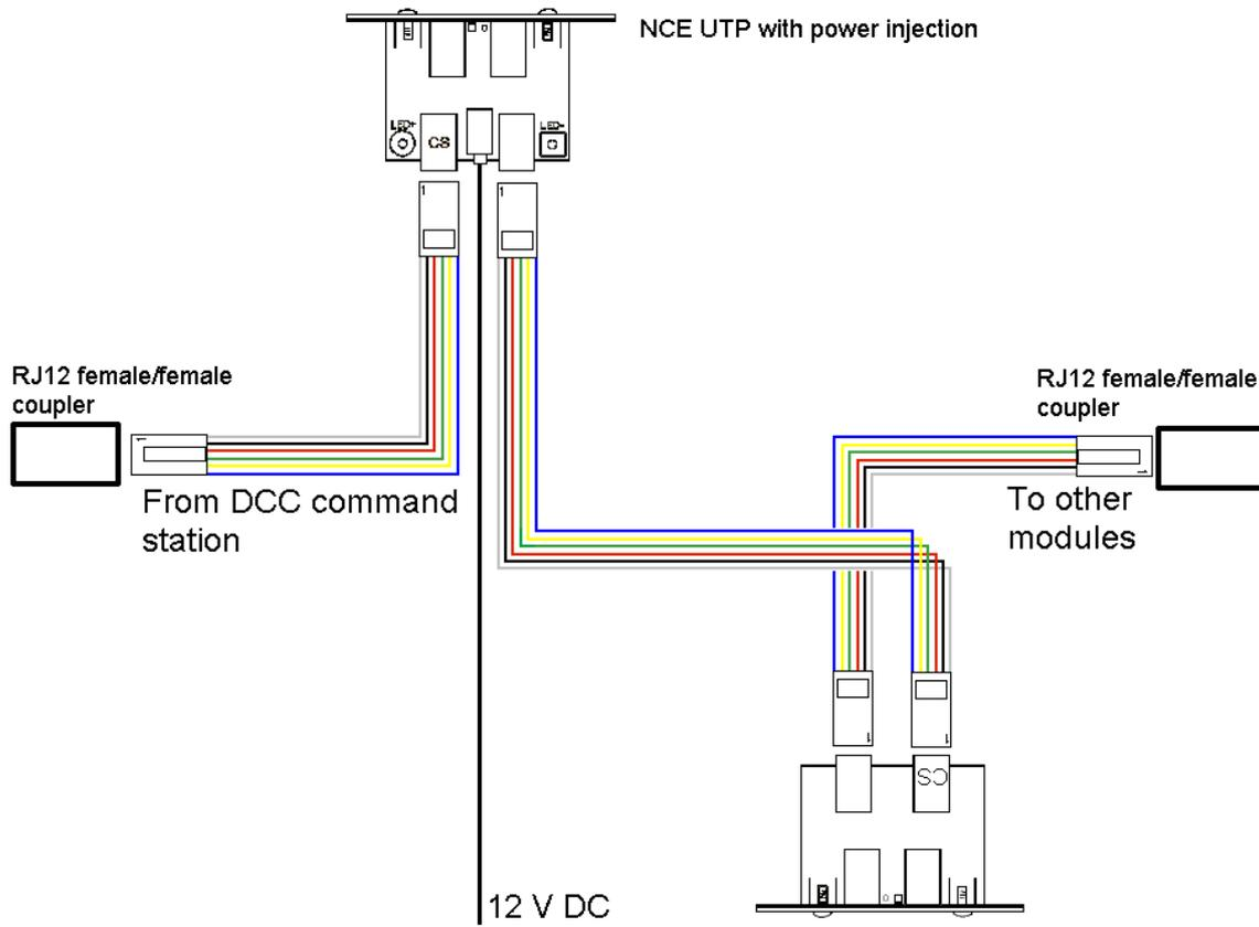
Figure 12: Wiring path for DCC command bus with power injection for NCE or SystemOne
