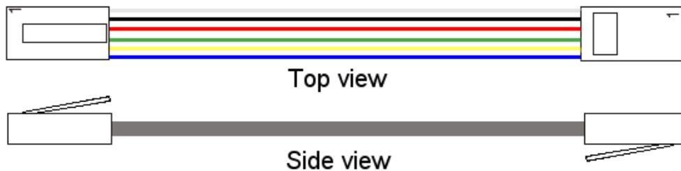
Figure 8: RJ12 straight through cable
