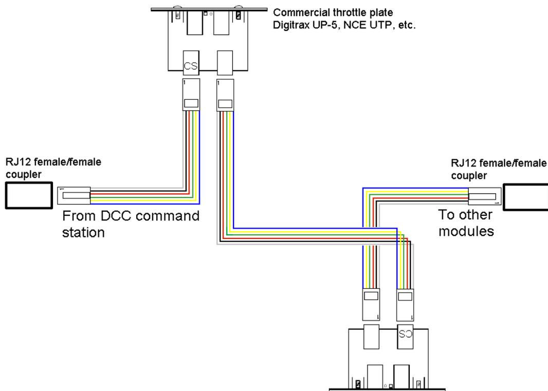
Figure 11: Wiring path for DCC command bus using commercial throttle jacks and RJ12 patch leads. Patch leads can be bought or home made.
